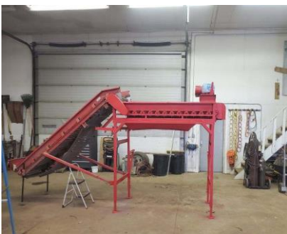
The brusher has been raised for easier cleanout and rollers were replaced
